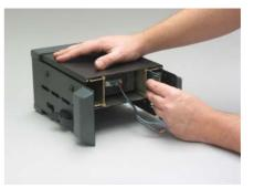
Grasp the PCB edge of the battery charger PCB and gently pull out
