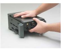
Grasp the front panel of the 2040 adaptor and gently pull away from the connectors
