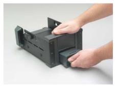
Remove the battery cartridge as shown
