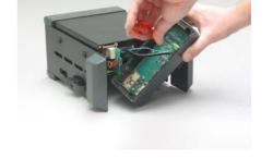
Using a flat blade screw driver remove the wires from the terminal block to the connector on the battery cartridge housing.
