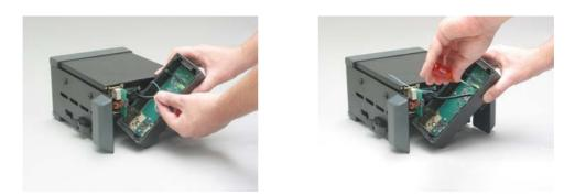
Note the location of the cables before disassembly to enable re-assembly
