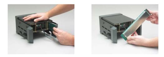
To access components on the battery charger PCB the RF shield must be un-soldered.
