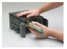
Grasp the PCB edge of the automatic antenna tuner PCB and slide out
